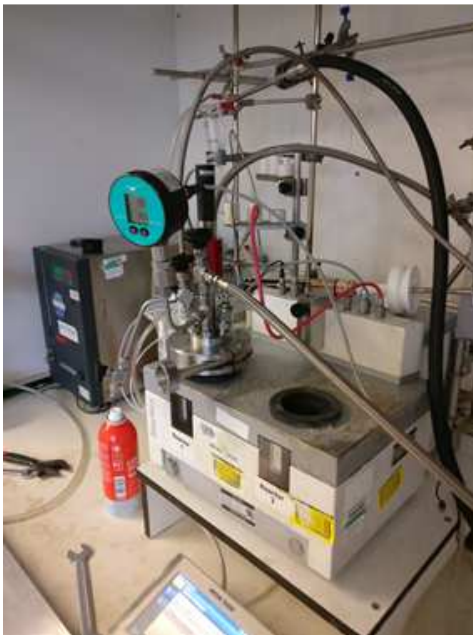
Figure 4.16: Hydrogenation of 1-(difluoromethyl)-4-nitrobenzene using an EasyMax reactor
