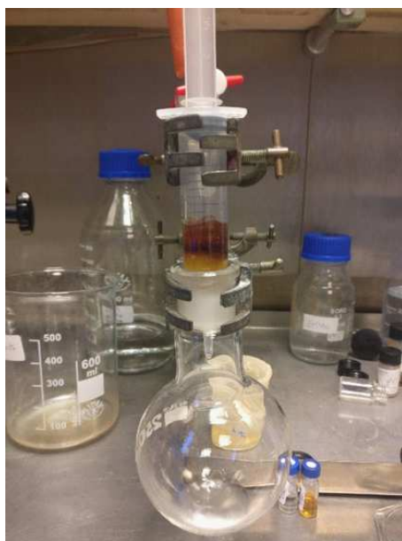
Figure 3.2: Small scale silica plug used to remove tar and HF without an aqueous workup to isolate compounds 96 and 96b-f
