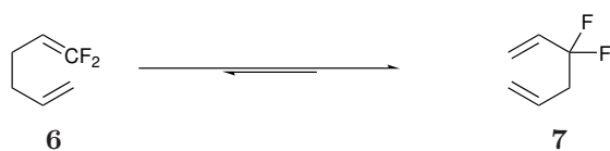
Figure 1.4: Isodemic Cope rearrangement of 6 illustrating the preference for fluorine to bond to an sp^3 carbon
