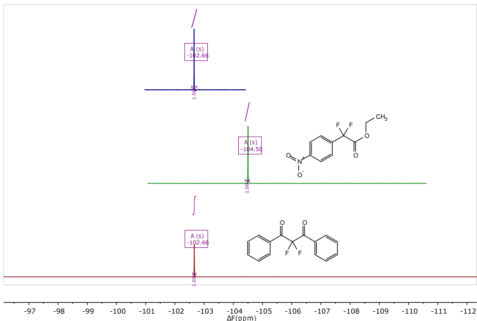
Figure 4.12: ^{19}\text{F} NMR spectra of the crude product post aqueous workup up (top) and reference spectra of ethyl 2,2-difluoro-2-(4-nitrophenyl)acetate (middle) and 2,2-difluoro-1,3-diphenylpropane-1,3-dione (bottom)
