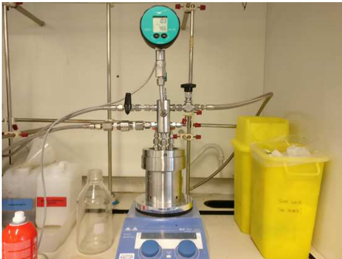
Scheme 4.20: Catalyst screening for the hydrogenation of ethyl 2,2-difluoro-2-(4-nitrophenyl)acetate using a Cat24 hydrogenation reactor
