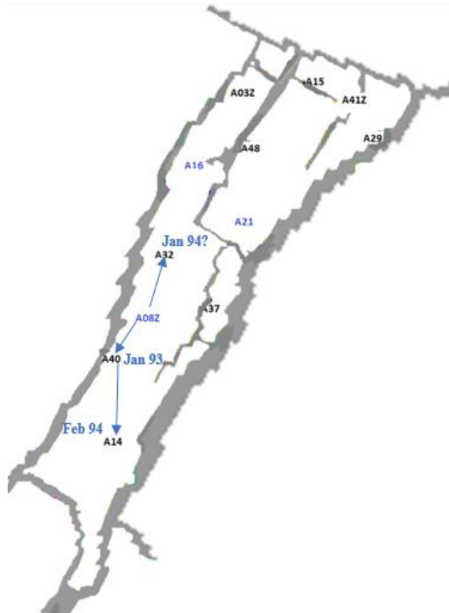
Figure 96- Water Injection Paths of A08Z, with Water Breakthrough Dates
