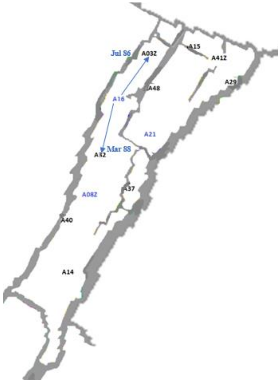
Figure 98- Water Injection Paths of A16, with Water Breakthrough Dates
