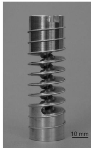
Figure 6.3 : Photograph of a superconducting wire mounted on a tee-shaped Walters spring. S_T = 6.35 mm, R_{Maj} = 12.5 mm. Figure taken from Ref. [37]
