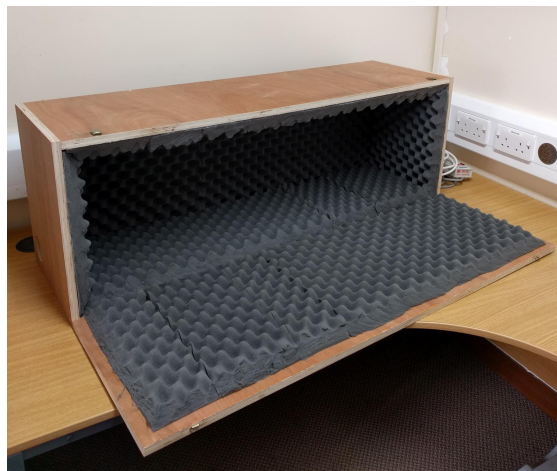
Fig. 4.1: The constructed MDF chamber with appropriate soundproofing inserts; each soundproofing insert has a self-adhesive backing.
