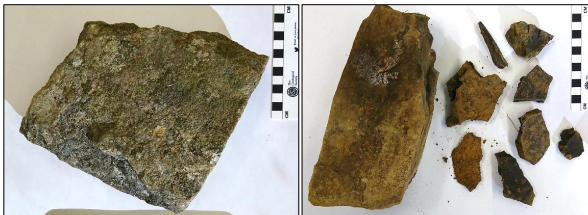
Figure 2.8: Outcrop samples of OC 1 (Hazelhurst Fell, Pendle Grit (left)) and OC 7 (Wolf Fell, Upper Bowland Shale (right)) before removal of any weathered surfaces.
