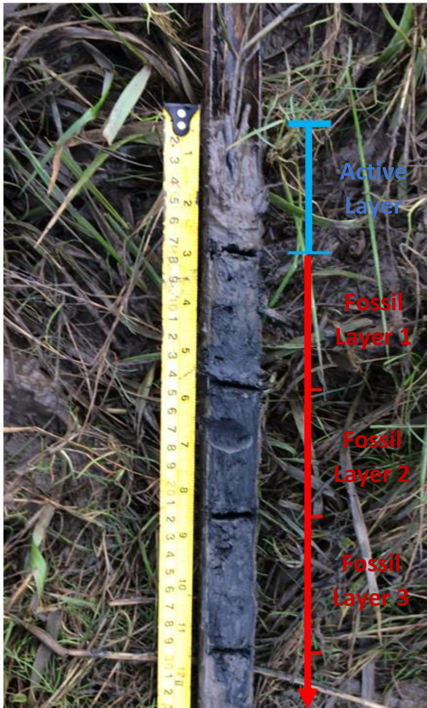
Figure 4.6. Test stratigraphy from Marsh B. The active layer (light blue) is clearly distinguishable due to its higher organic content, light brown colour and clear connection to the above-ground vegetation. Alternatively, the fossil layers (red) show no clear connection to the above-ground vegetation and have a lower organic content.
