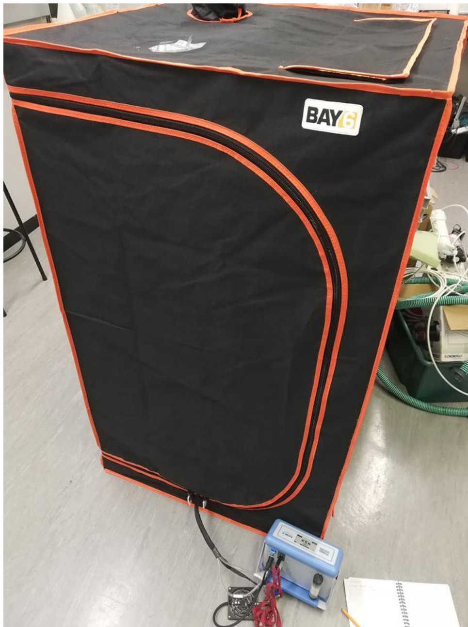
Figure 3.3[b]: Growth tent closed for measurement of gaseous flux under light conditions as shown in [a]. EGM-5 remains on outside of tent connected to CPY-5 on inside.
