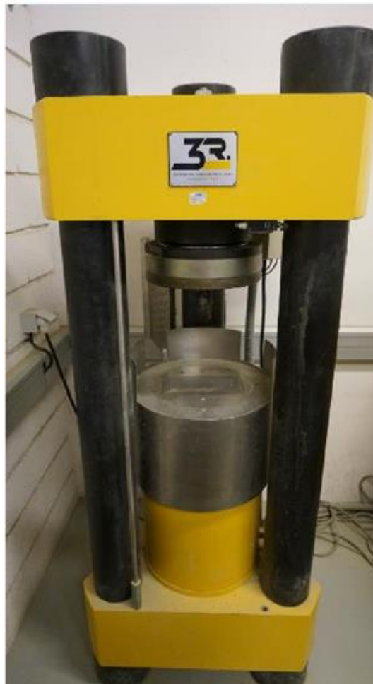
Figure 4.10: 3R RP 3000 TC/TH press with a load capacity of 3000 kN (from Bruno, 2016).
