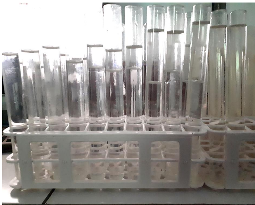
Figure 6.11: Visual examination of test-tubes after 72 hours from the addition of urea and calcium chloride in distilled water (equimolar urea and calcium chloride concentrations varying from 0.010 mol/L to 4 mol/L).
