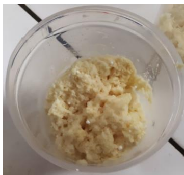
Figure 6.15: Formation of a semi-liquid paste after addition of calcium chloride to test-tubes containing distilled water, soybeans powder and urea (urea/calcium chloride concentration of 2.50 mol/L).
