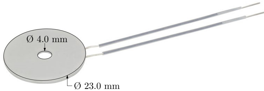
Figure 3.3 | Photograph showing the dimensions of the ceramic heater. One heater is placed either side of the vapour cell, heating it to \sim 125^{\circ}\text{C} to provide a sufficient optical depth for the probe.
