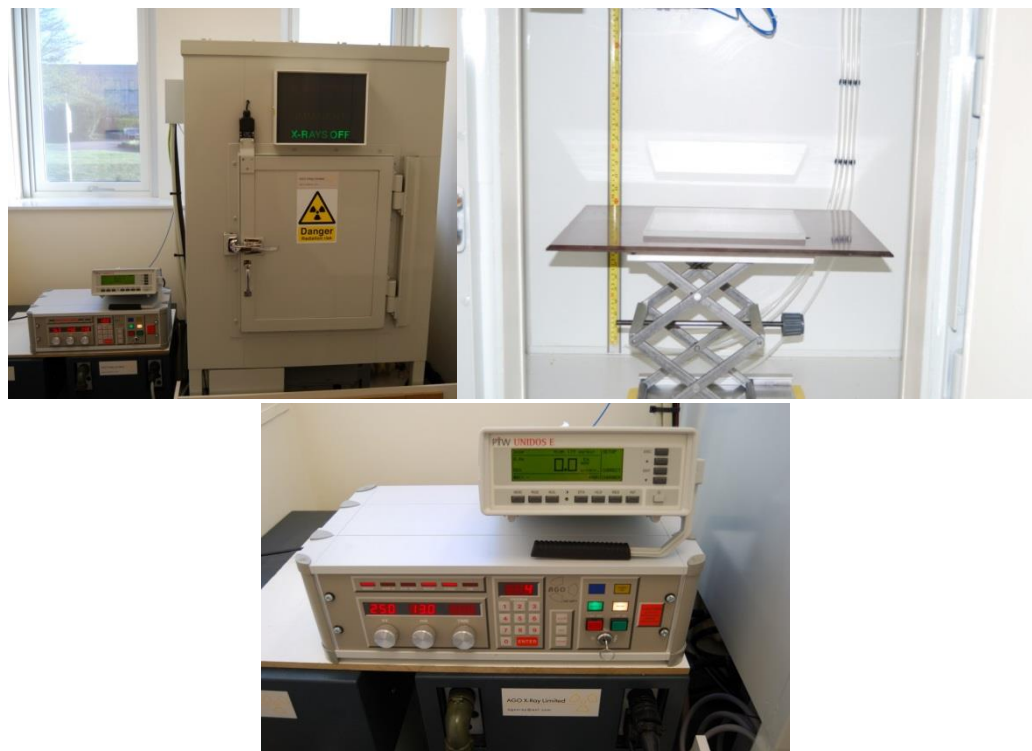
Figure 2.3: 250 kVp X-ray unit (CD160/1, AGO X-ray Ltd, Martock UK) located at PHE, Chilton (UK) where all x-irradiations were performed
