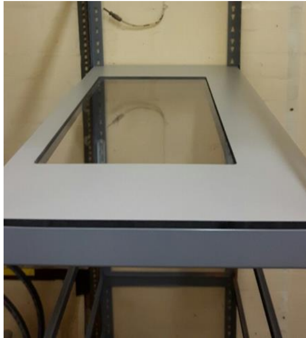
Figure 2.5: Wooden shelf used during exposures. The shelf had a Perspex 'window' on which the Corex exposure boxes were placed. The shelf could be moved to slot into the various shelf brackets to achieve the different dose-rates.
