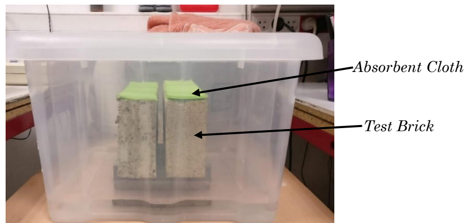
Figure. 5.9. Test Setup for Contact test
