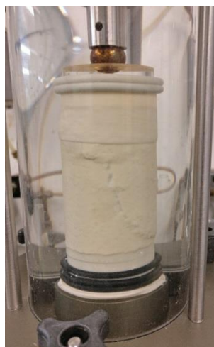
Figure 4.14. Typical setup for triaxial test
