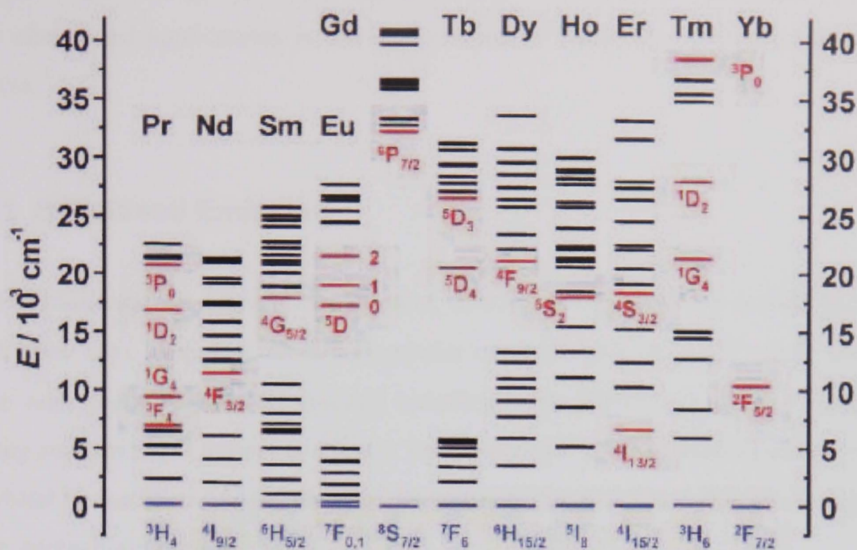
Figure 1. 1 - Partial energy diagram for the lanthanide aqua ions. Red lines indicate the main emissive levels, blue lines the ground state.
