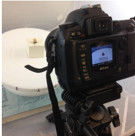
Figure 4.3. The equipment setup used to photograph tooth samples to be processed for 3-D photogrammetry models.
