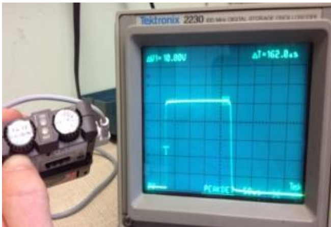
Figure 24 Re-calibrating the external voltage amplitude dial A
