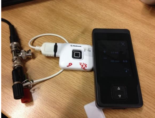
Figure 26 Verify ENS, controller and circuit with simulated tissue load to oscilloscope
