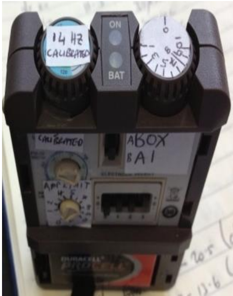
Figure 25 A model 3625 test stimulator with fully re-calibrated frequency, pulse width and voltage amplitude dials.
