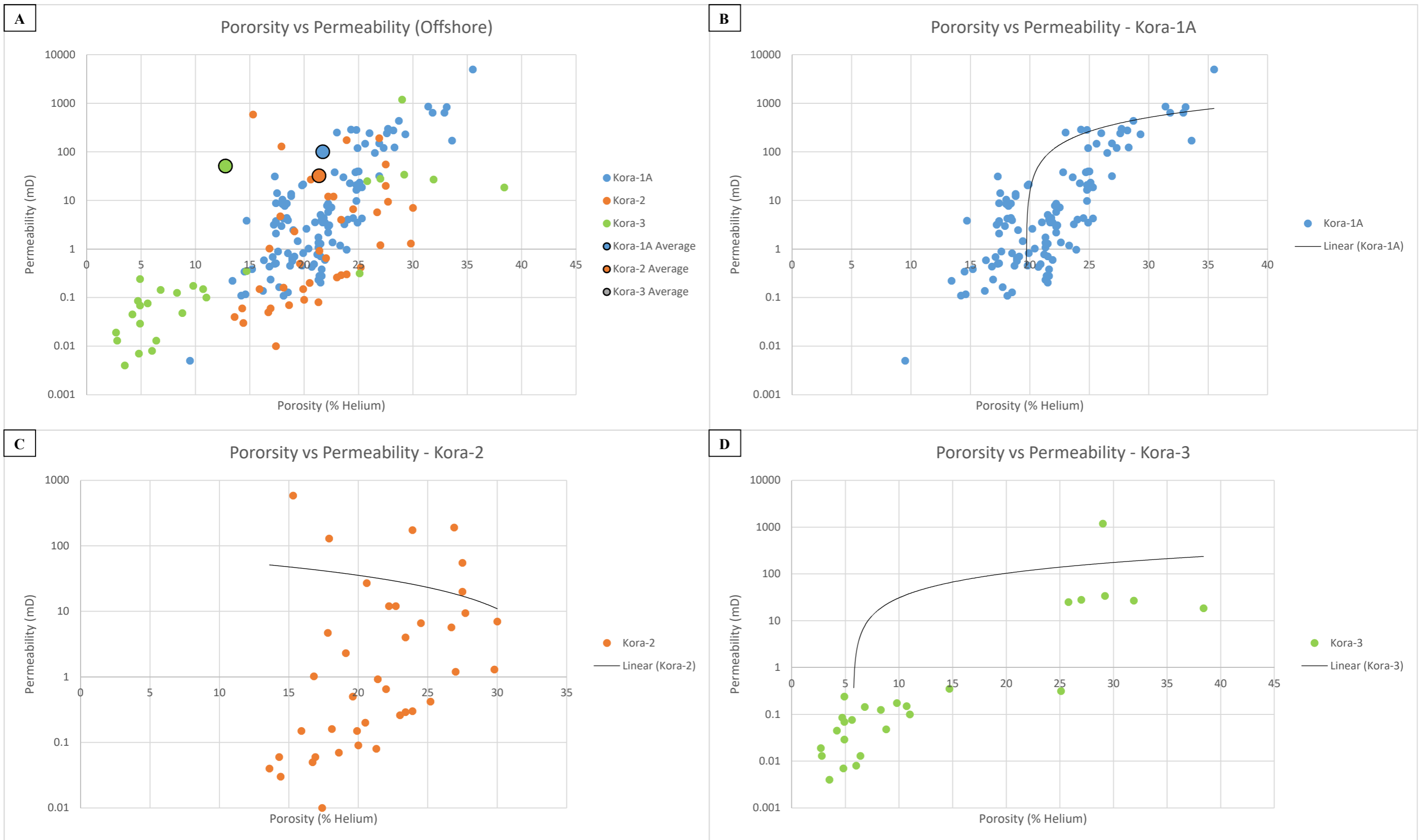
Figure 3.17: A collection of graphs where porosity is plotted against permeability for each well and for all the wells plotted together. A) A graph of helium porosity plotted against permeability for Kora-1A, Kora-2 and Kora-3 wells. B) A graph of helium porosity plotted against permeability for the Kora-1A well. C) A graph of helium porosity plotted against permeability for the Kora-2 well. D) A graph of helium porosity plotted against permeability for the Kora-3 well. All of these graphs have a linear trend line to supplement them, and this provides a an additional feature by which the difference between the average values at each end of the graph can be judged. It is also key to note that the graphs are logarithmic.
