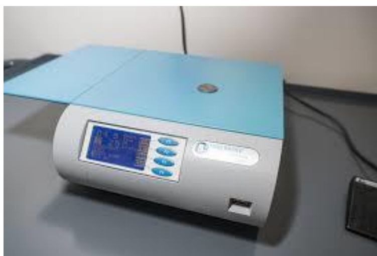
Figure 2.2: Tail-flick test (radiant heat) apparatus. Radiant heat is generated from an infrared source (50W bulb). This system can automatically start/stop timing when the mouse tail-flicks. When the mouse feels pain and flicks its tail, a sensor detects it, stops the timer and switches off the bulb. The reaction time of the mouse in s is determined and automatically recorded (Ugo Basile, Italy).
