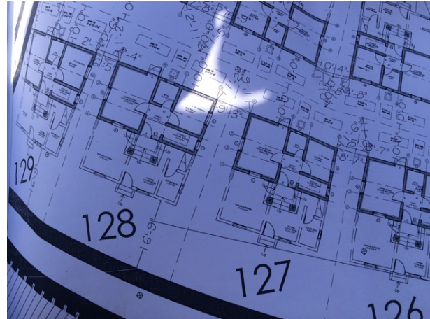
Figure 43.a (left) This plan shows the how the space is divided by the centralised entrance and corridor which leads to the two rooms on the side. Figure 43.b. (right) Photograph of CAD drawing of resettlement housing scheme taken at Danyore Site.
