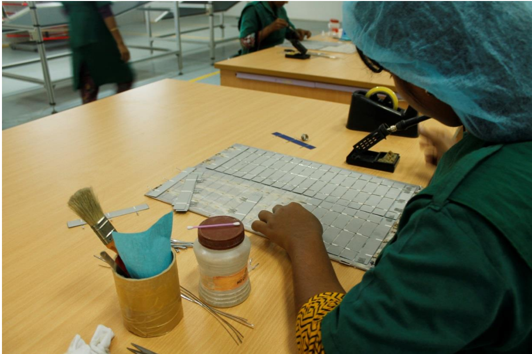
Figure 9:1 Assembling a solar panel
