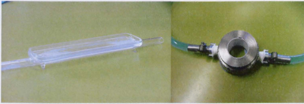
Figure 3.15 Left: Quartz glass trough, designed as shallow as possible to prevent thermal gradient over trough depth. Right: Aluminium PTFE-lined trough, cooled from sides and with glass base to enable microscopy
