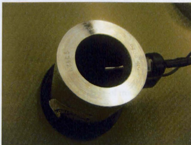
Figure 3.13 UVM sample cell, the temperature probe can be seen protruding from cell wall.
