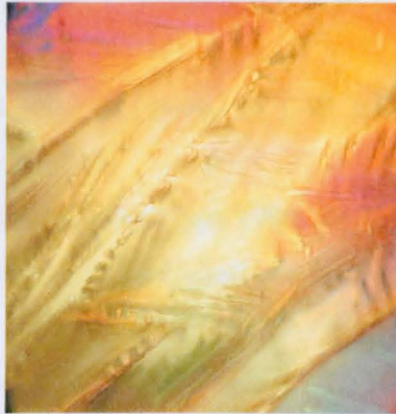
Figure 3.16 Water freezing from the surface, nucleated by heptacosanol, in quartz glass trough. 10x magnification, cross-polarisers and 539nm tint plate used to enhance image
