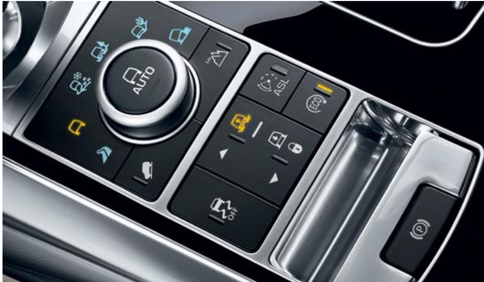
Figure 1.2 The terrain response selector in a modern Land Rover vehicle, including 'Auto' mode which relies on mechanical sensors to identify terrain type.
