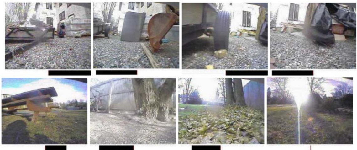
Figure 2.13 Example images from the data used to test DAVE [39]. The black bars represent predicted steering direction and magnitude.
