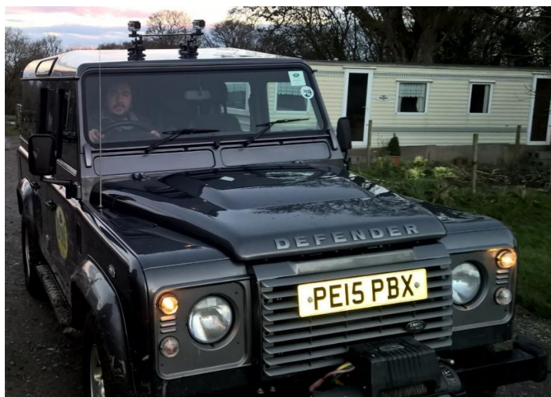
Figure 5.5 An off-road vehicle being driven as part of our data collection process. A stereoscopic camera rig attached to the roof of the vehicle was used to capture data in a wide variety of off-road environments.
