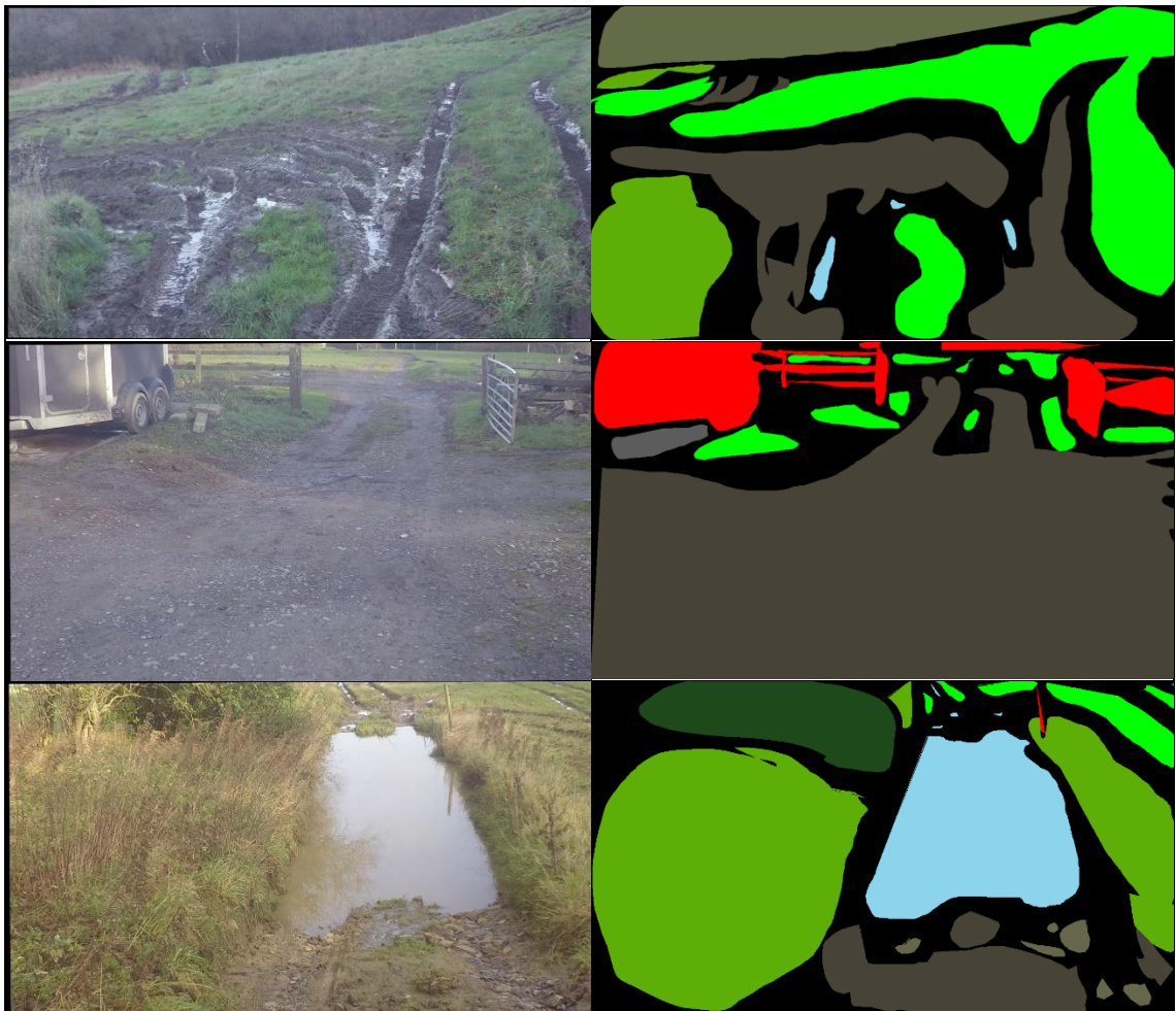
Figure 3.4 Example images from our off-road data set along with corresponding partially labelled ground truth
