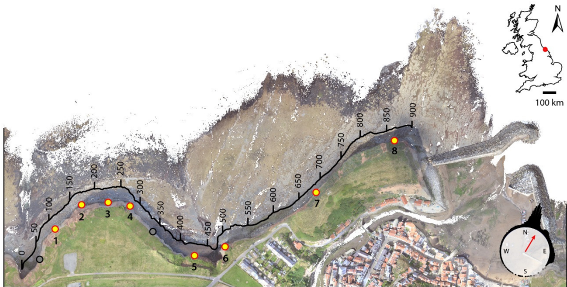
Figure 5.02 Accelerometer installation sites west of the village of Staithes, North Yorkshire, plotted on top of a point cloud obtained in August 2014. Grey/yellow markers denote un/successful installations. Inset: circular histogram of wave directions recorded over the monitoring period, with the mean marked in red.
