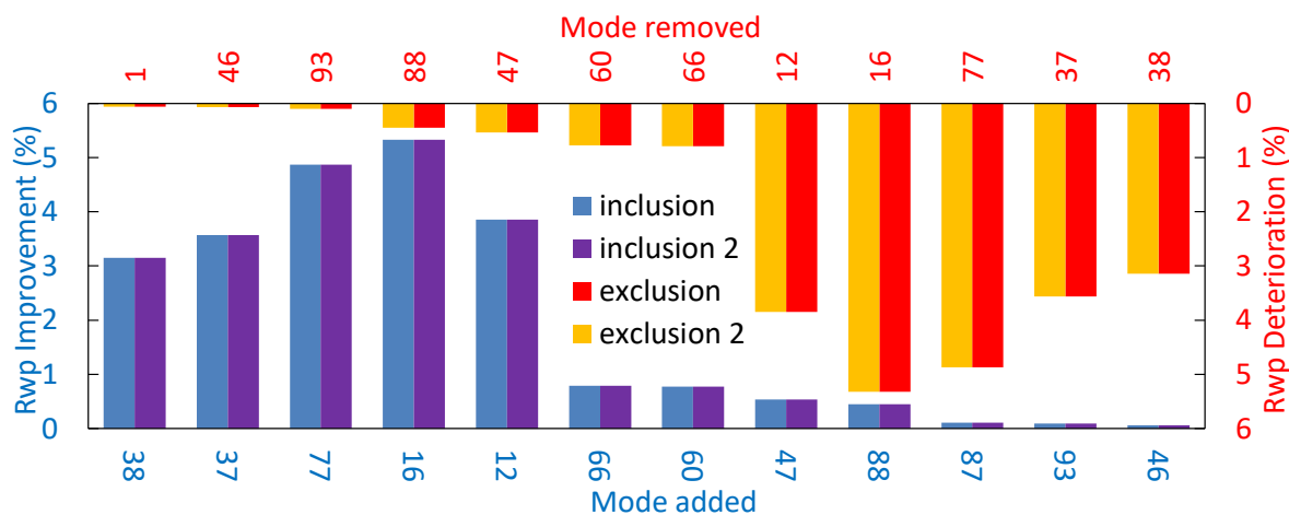
Figure 2.36: Blue/Purple (left and bottom axes): Improvement in combined X-ray / TOF neutron R_{wp} on successive inclusion of 12 highest ranking distortion modes. Red/Orange (right and top axes): Deterioration in R_{wp} on successive exclusion of 12 highest ranking distortion modes.
