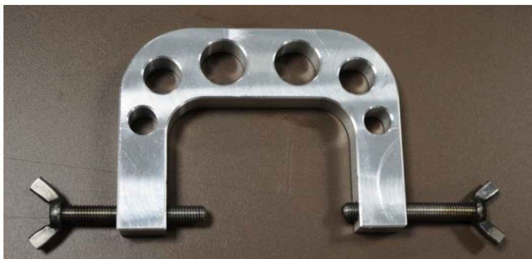
Figure 4.34: Vice attachment made to drive slave pistons
