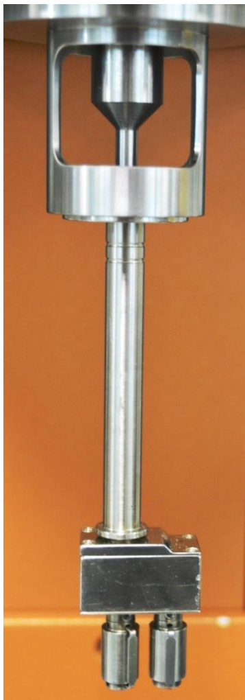
Figure 1.6: Sentmanat extensional rheometer attachment
