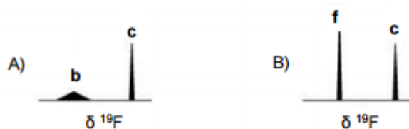
Figure 24 Illustration of the line-broadening effect, where b = bound molecule, f = free molecule and c = control molecule in A) presence of protein and B) absence of protein
