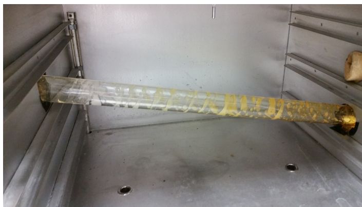
Fig. 14.10 Photograph of a helix formed by the reactants travelling down the work-tube as it rotates.
