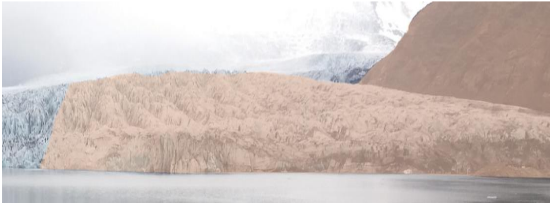
Figure 4.3) The coverage of the scan program which automatically scanned once every hour. The area includes the glacier ice directly in front of the scanner and the area of bedrock to the right but does not extend further to the left of the image. This is because the point density was greatly reduced in this area due to an embayment in the glacier terminus where the ice is beyond the maximum measurement range of the VZ-4000.
