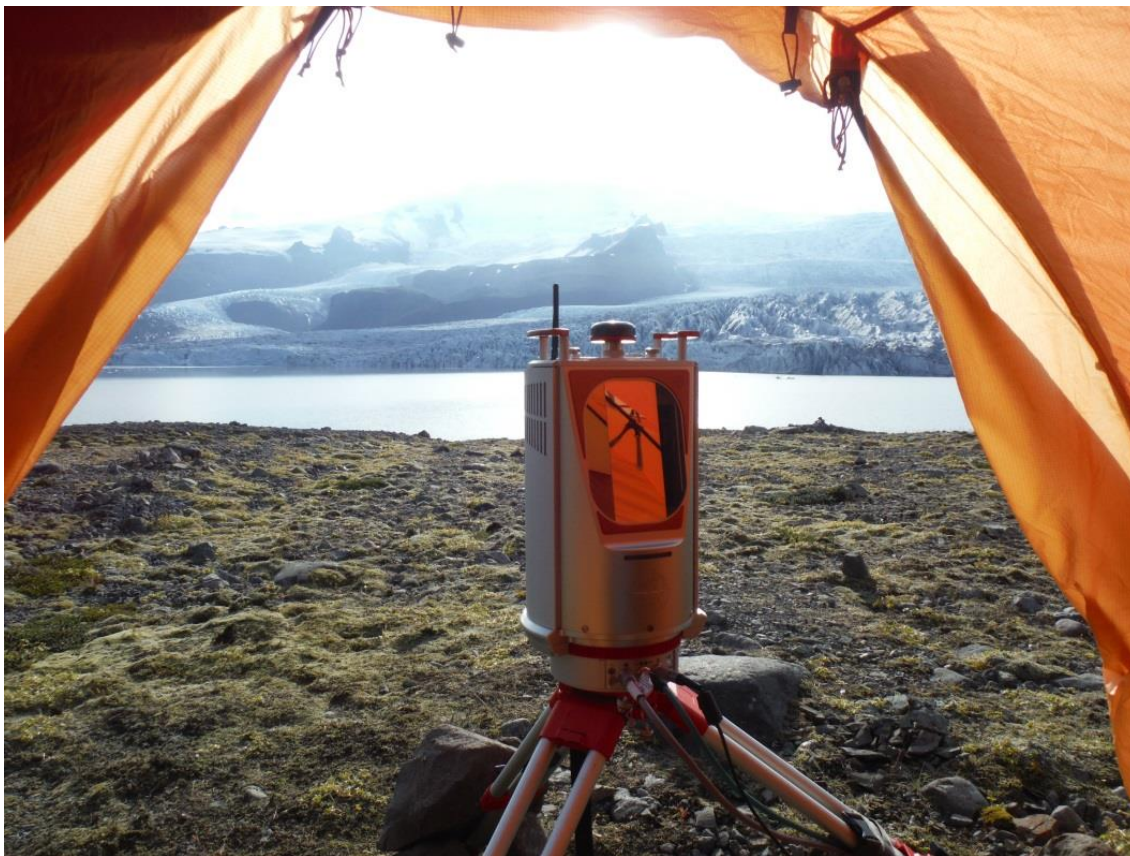
Figure 4.4) The location of VZ-4000 in front of Fjallsjökull under the tent porch to provide some shelter from wind and rain.
