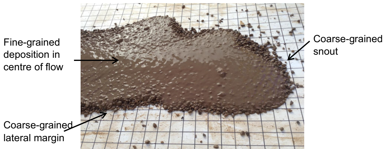
Figure 3.16. Image of a debris flow deposit generated during a rigid-bed experiment, demonstrating some key characteristics of natural debris-flow deposits.
