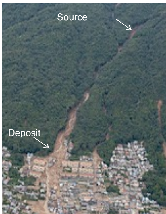
Figure 1.1. Photograph of the Midori-ga-oka debris flow, one of 107 debris flows which were initiated in Japan on 20 th August, 2014 in response to high-intensity rainfall, causing infrastructural damage and loss of life. (Wang et al., 2015).
