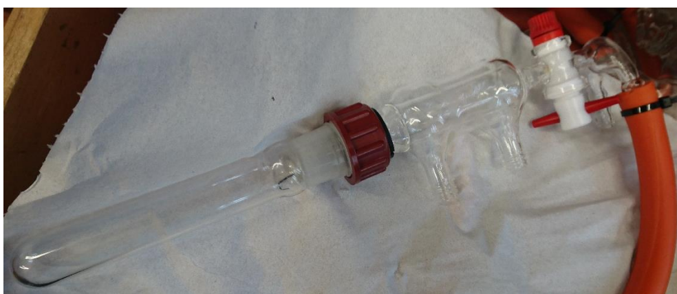
Figure 2.20. Photograph of a single reactor used in the carousel reactor system.
