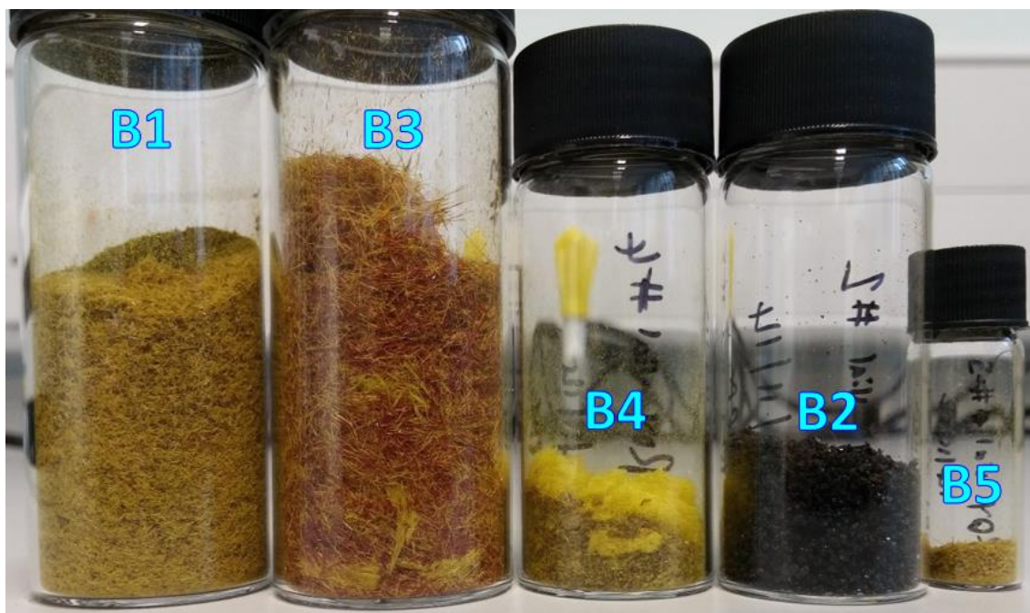
Figure 4.6 Synthesised ROY in vials. Each batch was collected from consecutive crystallisations from the one synthesis. The batches are, from left to right: one, three, four, two and five.
