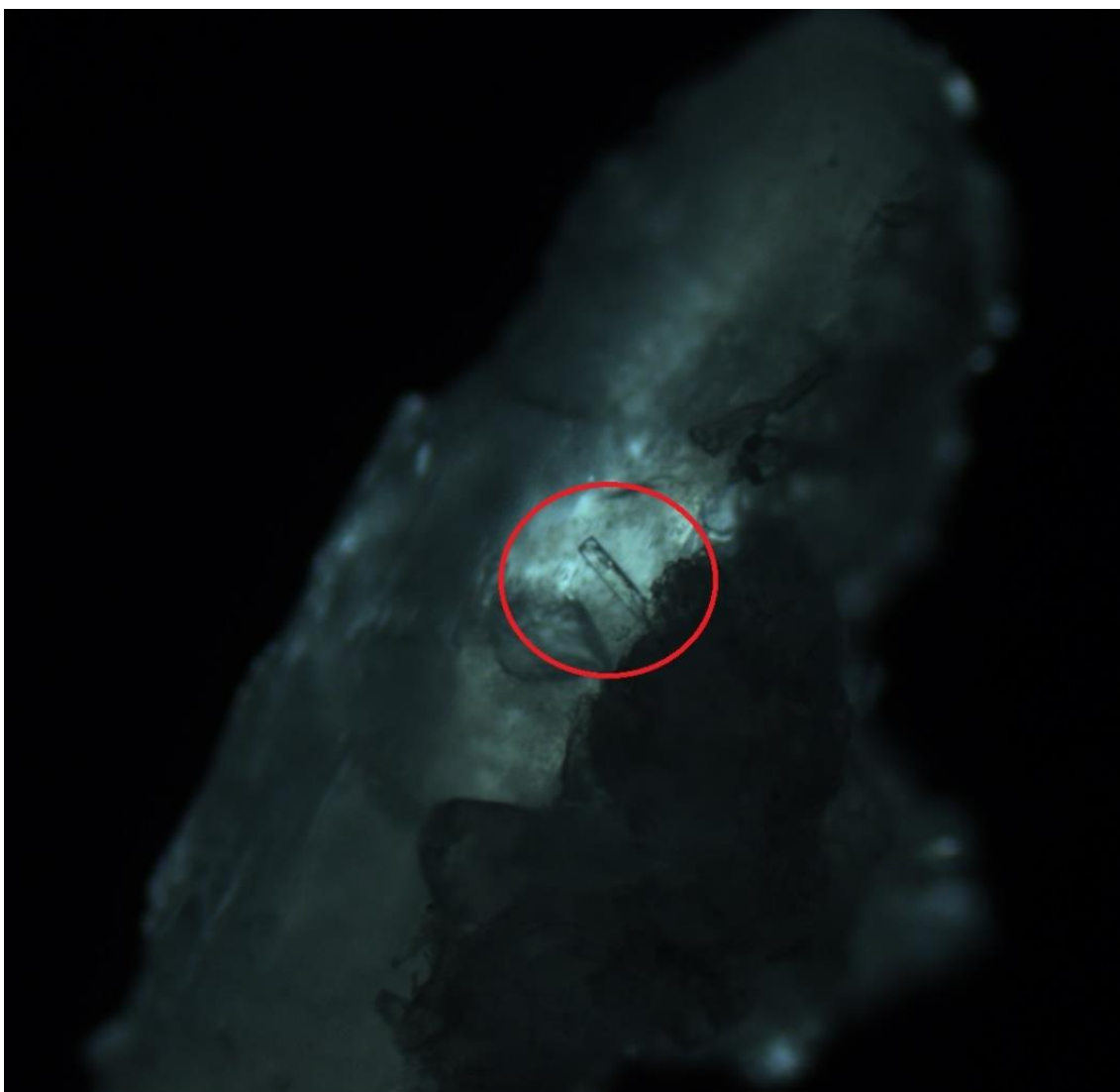
Figure 6.16 Micrograph of a single crystal of ornidazole:5-nitroisophthalic acid (circled) on a larger crystalline mass viewed under cross polarised light.
