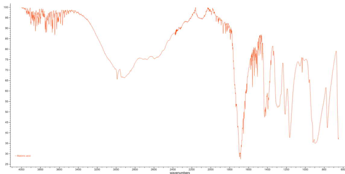
Figure 2. Infrared spectrum of malonic acid.
