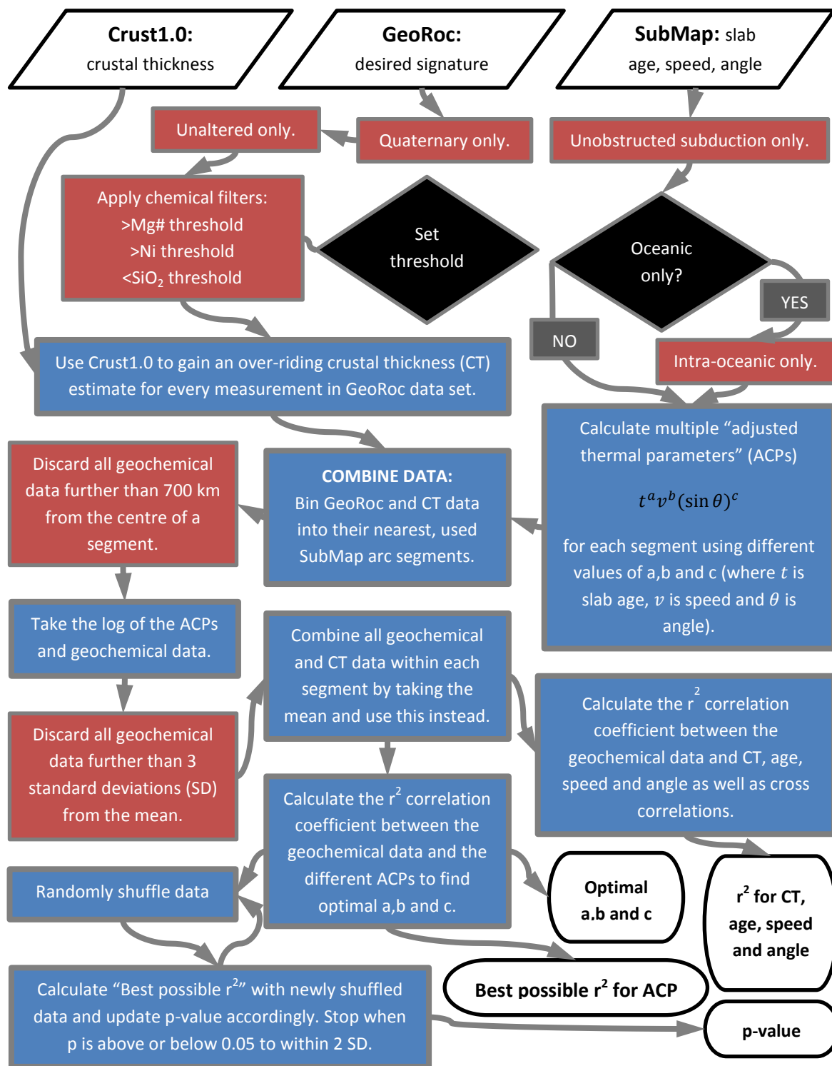
Figure 4.3 Flow chart summary of the processing on the GeoRoc, Submap and Crust1.0 databases to arrive at the data presented in the Results section of this chapter. This is described more fully in the main text. Data inputs are in white parallelograms, user inputs are in black diamonds, filtering steps are in red boxes, other steps are in blue boxes, and the outputs are in white rounded boxes.
