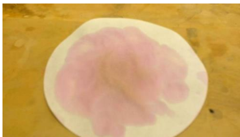
Figure 4.13 – Cobalt (II) nitrate test for aluminium in polymer 10
