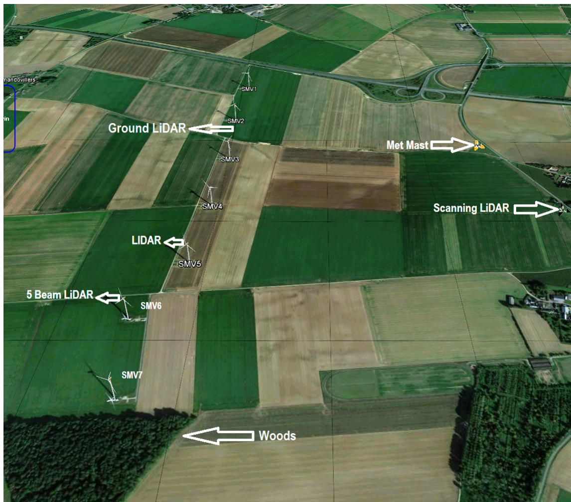
Figure 6.3 SMV layout and surrounding with positions of met mast and LiDAR [187]
