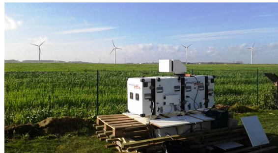
Figure 6.5 Scanning LiDAR 1.2km east of SMV for horizontal and vertical scans
