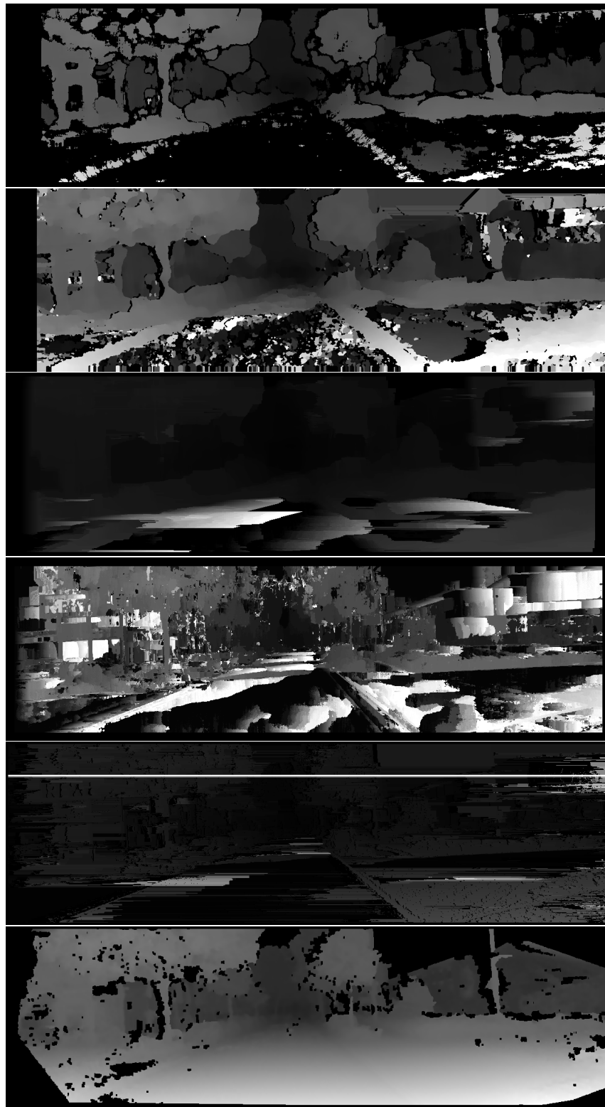
Figure A.1: Dense stereo disparity maps generated using the KITTI data. Algorithms used, top to bottom: BM, SGBM, NoMD, Cross, AdaptDP, ELAS.
