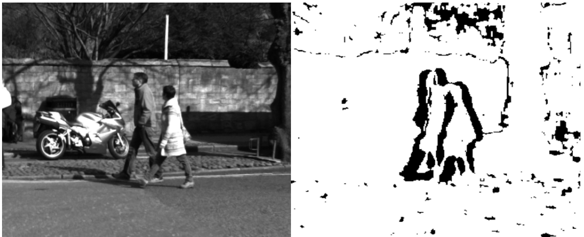
Figure 5.4: Left: Intensity image from left stereo camera. Right: Threshold of disparity difference image or DMM.
