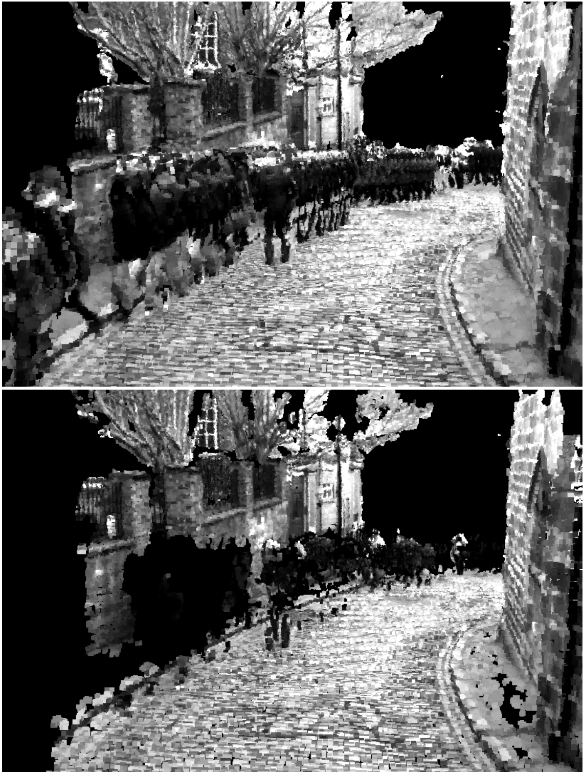
Figure 5.10: Top: Large group of people moving at various speeds including some static bystanders. Bottom: Pedestrians are largely removed, elements that remained static between frames are still present.
