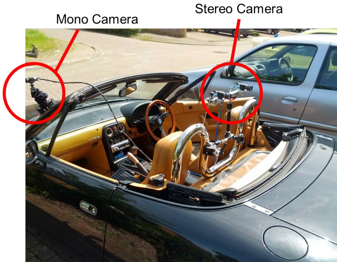
Figure A.17: The next data capture phase saw the addition of side-facing cameras and the mounting on a vehicle to reduce the effect rough surfaces. The cameras were also upgraded to global shutters to eliminate integration artifacts due to rolling shutter.
