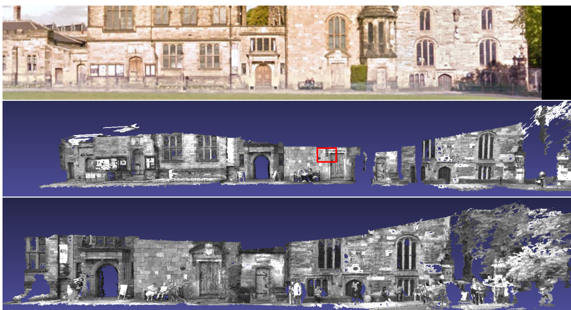
Figure 6.5: Top: Image from Google Earth [1]. Middle: Point cloud from SfM reconstruction viewed using Meshlab [6] (9.7 million points). Bottom: Same location captured an hour later with more stationary pedestrians present (11.2 million points).
