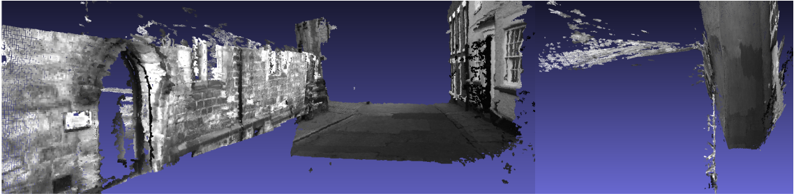
Figure 6.13: Left: Ground level view of aligned reconstruction. Right: Birdseye view of the same combined point cloud.
