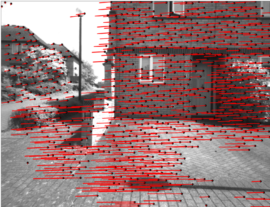
Figure 4.5: Features tracked using sparse optical flow. Black dot indicates the feature point start location, Red line indicates direction and magnitude of motion.
