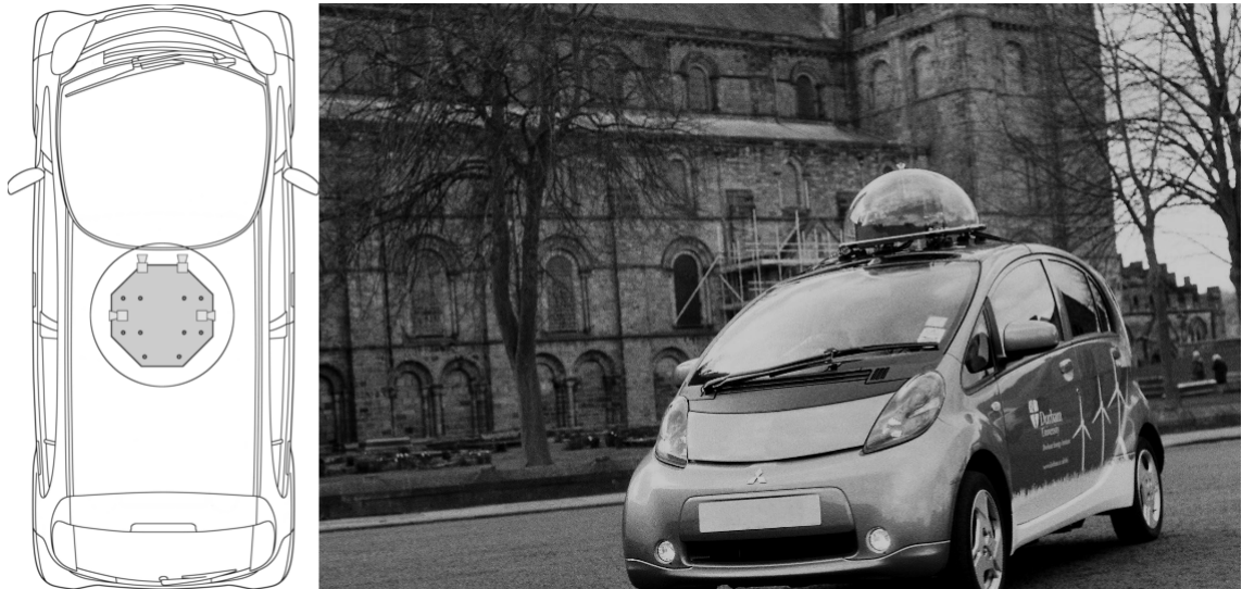
Figure 4.2: Data logging pod mounted on our Mitsubishi i-MiEV electric vehicle. Left, schematic view from above. Right, Parked near Durham Cathedral, the site of many of our data collection activities.
