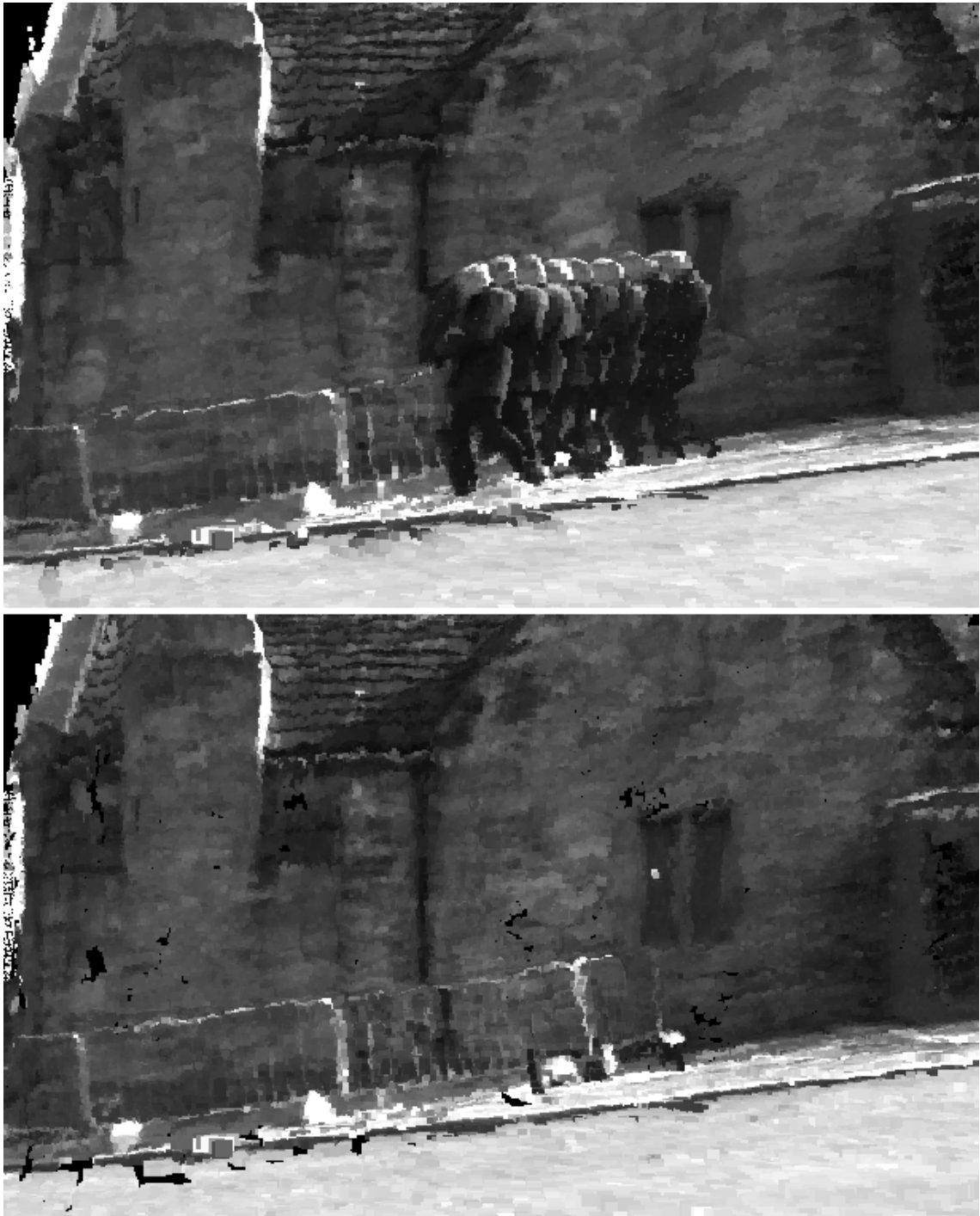
Figure 5.9: Top: A slow moving pedestrian with approximately 50% self-overlap between frames. Bottom: Successfully removed from mapping solution.
