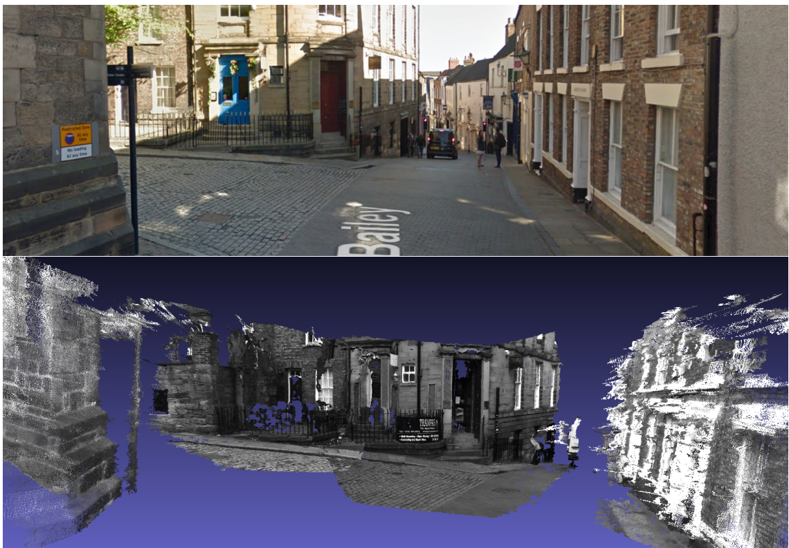
Figure 6.12: Top: Google Street View [7] image showing the North Bailey location. Bottom: Reconstruction from 3 non-overlapping views auto-aligned.
