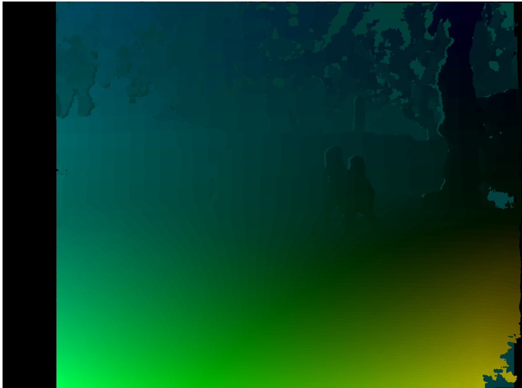
Figure 5.5: Flow from disparity of the illustrated failure mode in Figure 5.4 with the vehicle driving forwards and right (flow direction and magnitude are represented respectively by the hue and value channels of the HSV colour space).
