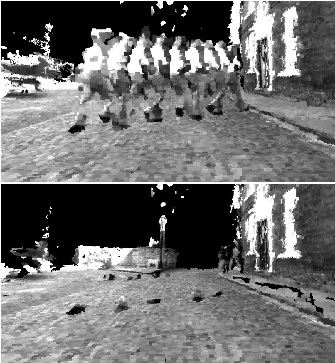
Figure 5.11: Top: Fast moving pedestrian with motion perpendicular to camera motion. Bottom: Successful removal of moving components, however the feet remain visible in the point cloud as these are temporarily static during contact with the ground. The motion of the leg above the ankle has been successfully removed.
