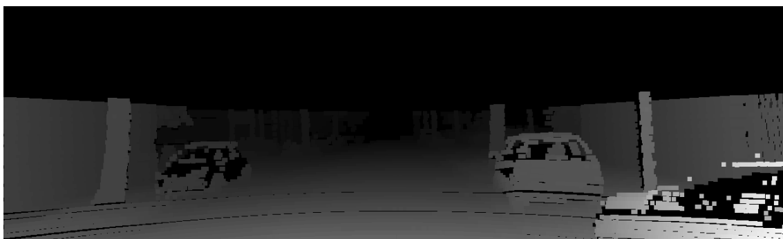
Figure 2.1: Example of KITTI laser scanner data projected into the left greyscale-camera coordinate system and scaled to simulate a disparity map.
