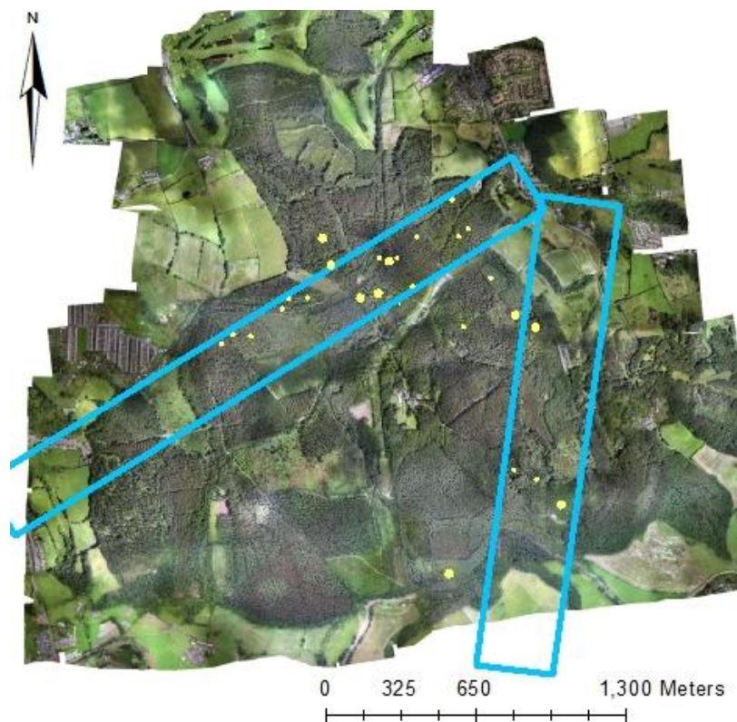
Figure 4. Orthomosaic captured July 2009 during the first LiDAR acquisition. LiDAR data from the 2011 survey is only available within the blue boundaries whereas LiDAR data from the 2009 survey is available across the entire forest. Yellow circles represent all Chopwell Woodland field data sample plots available from the Ozdemir and Donoghue (2013) study.
