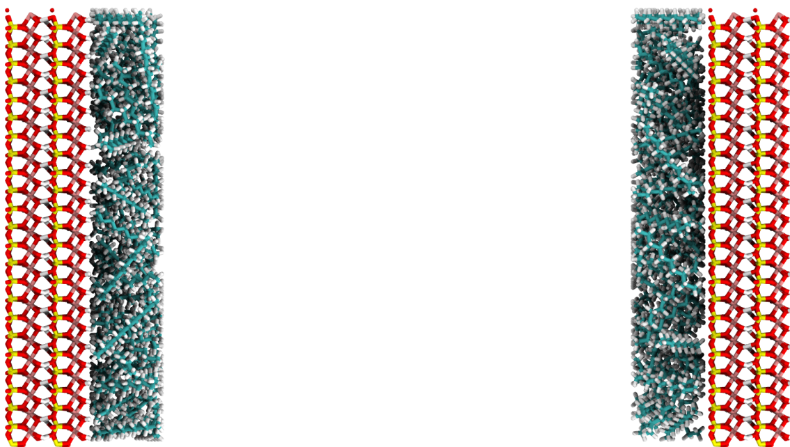
Figure 5.4: A snapshot showing the initial model of decane interacting with kaolinite before water is added. The PackMol software package 24 has been used to create the densely packed organic phase adjacent to the siloxane and hydroxyl surfaces. All simulations start with similar configurations. The clay structure contains the same color scheme as in Figure 5.3, whilst the oil molecules contain carbon (blue) and hydrogen (white).
