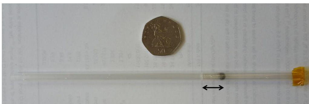
Figure 2.12. Sample setup for SQUID magnetometry, showing the black \text{Ce}_2\text{O}_2\text{ZnSe}_2 sample within the gelatin capsule (marked by a double headed arrow), within the straw.
