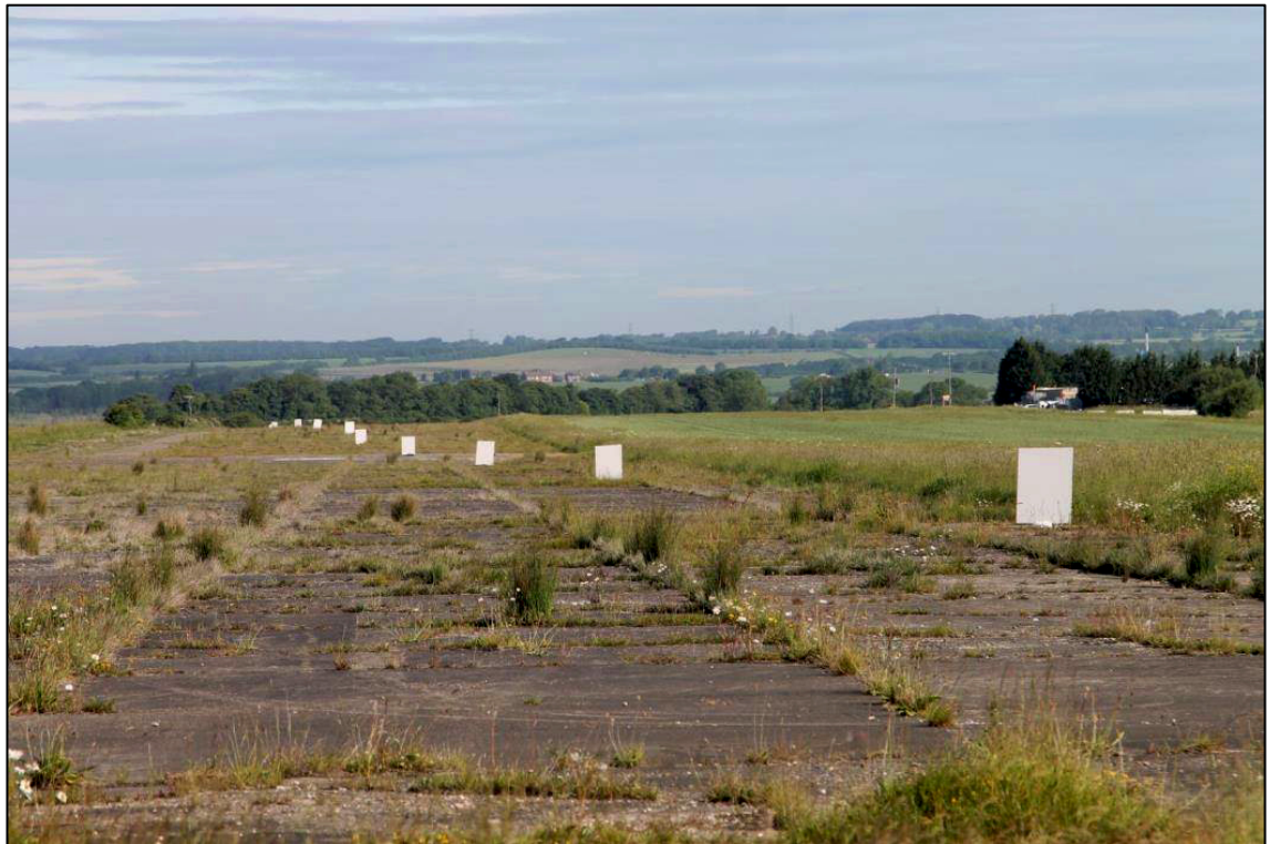
Figure A.E.3: Targets distributed at 100 m intervals between 100 m and 1,000 m on a disused former WWII airfield. The targets were repeatedly scanned at 30 minute intervals over a 24 h period.
