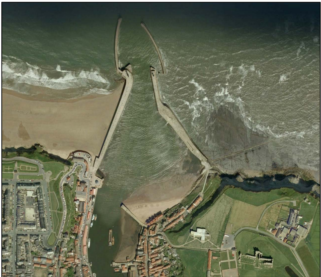
Figure 3.2: Infoterra aerial imagery of Whitby (2009), acquired from Google Earth within the same area as Figure 3.1. Here, the foreshore platform in front of East Cliff is partially inundated. Previous LiDAR surveys of the cliff have been undertaken from this platform. The scale here is the same as that applied in Figure 3.1.
