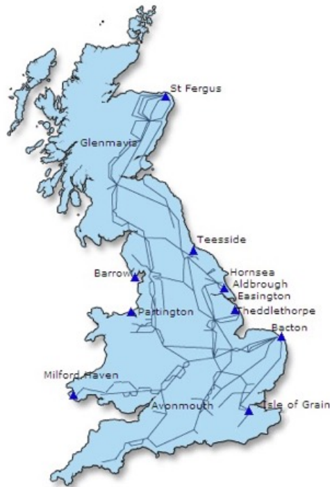
Figure 1 - Map of the UK National Transmission System, courtesy of National Grid 2015 (does not directly serve Northern Ireland – see footnote 11)
