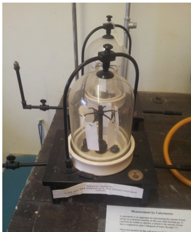
Figure 9 - Photograph of the apparatus used for detecting hydrogen sulphide in town gas (Fakenham Gas Museum, 2014)
