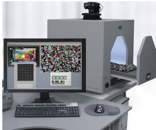
Figure 37 DigiEye equipment in use in P&G Newcastle, image taken from manufactures website 87
