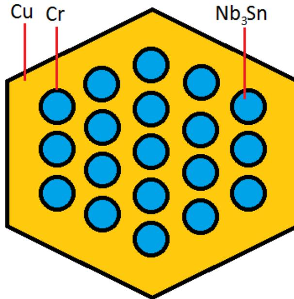
Figure 8.1: Schematic of one of the common structures for Nb<sub>3</sub>Sn wires.
