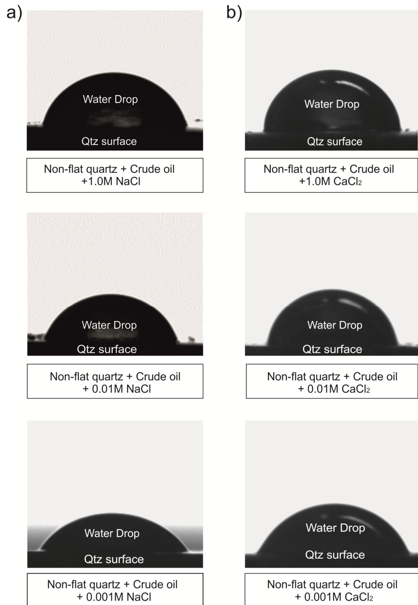
Figure 5.14: Contact angle images of water droplet on non-flat quartz surface at room temperature and pressure. a) Non-flat quartz aged in crude oil during exposed with various NaCl concentrations. b) Non-flat quartz aged in crude oil exposed with various CaCl 2 concentrations. These images were scaled up from the real size of 2.5 \pm 0.5 mm 2.5 \pm 0.5 mm.
