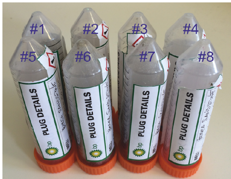
Figure 6.3: Sealed desaturated BST core plugs.
