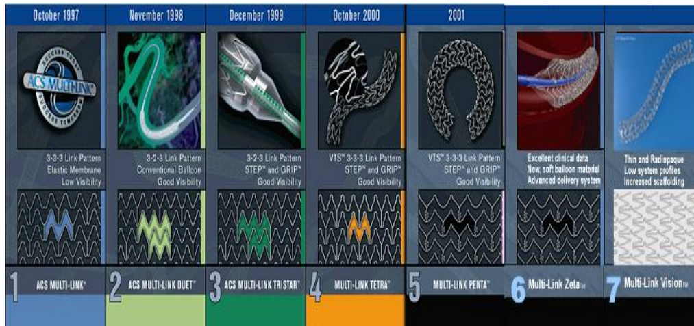
Figure 9. Evolution of the MULTI-LINK™ stent system. Reproduced with permission from Abbott Vascular company documents.
