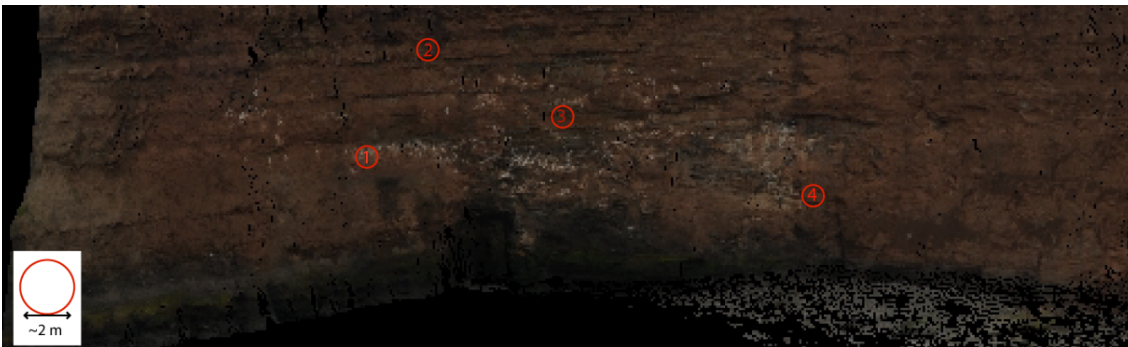
Figure 3.10: Images of the cliff sections (photographs draped over the point cloud in RiSCAN) used for uncertainty analysis: (a) flat section; (b) bay area. The numbers in red circles correspond to areas where depth change was measured – results are given in Table 3.3.
