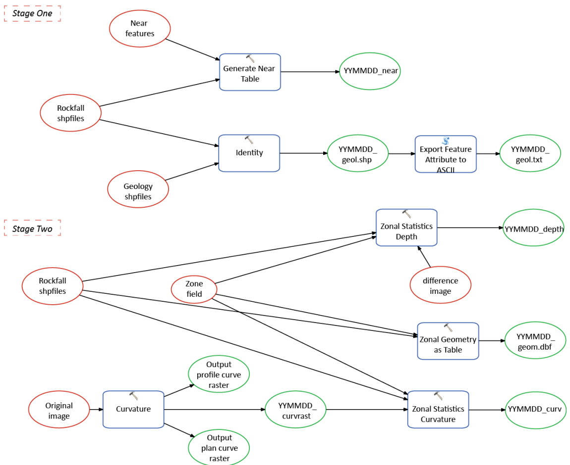
Figure 3.11: Workflow used for data analysis of the two year dataset: Red = inputs; Blue = Functions; Green = outputs.
