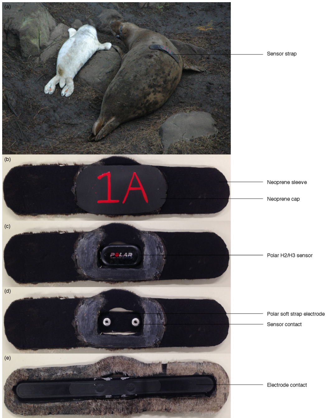
Figure 2.3. The sensor strap apparatus used to transmit RR intervals of female grey seals deployed in the field. (a) A grey seal female with a sensor strap containing a Polar ® H2/H3 sensor and Polar ® soft strap electrode on the Isle of May, Scotland. The sensor transmits RR interval data to the Polar ® RS800CX monitor (out of shot). Complete (b) and partially complete (c-e) sensor straps, post-retrieval, as viewed from above (b-d) and below (e) . See Figure 2.2. for full description.
