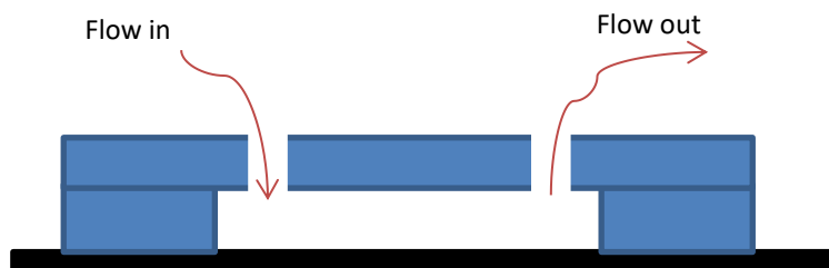
Figure 4.10 Structure of PDMS cell for fluorescence microscopy. The black shows a glass cover slip and the blue shows PDMS
