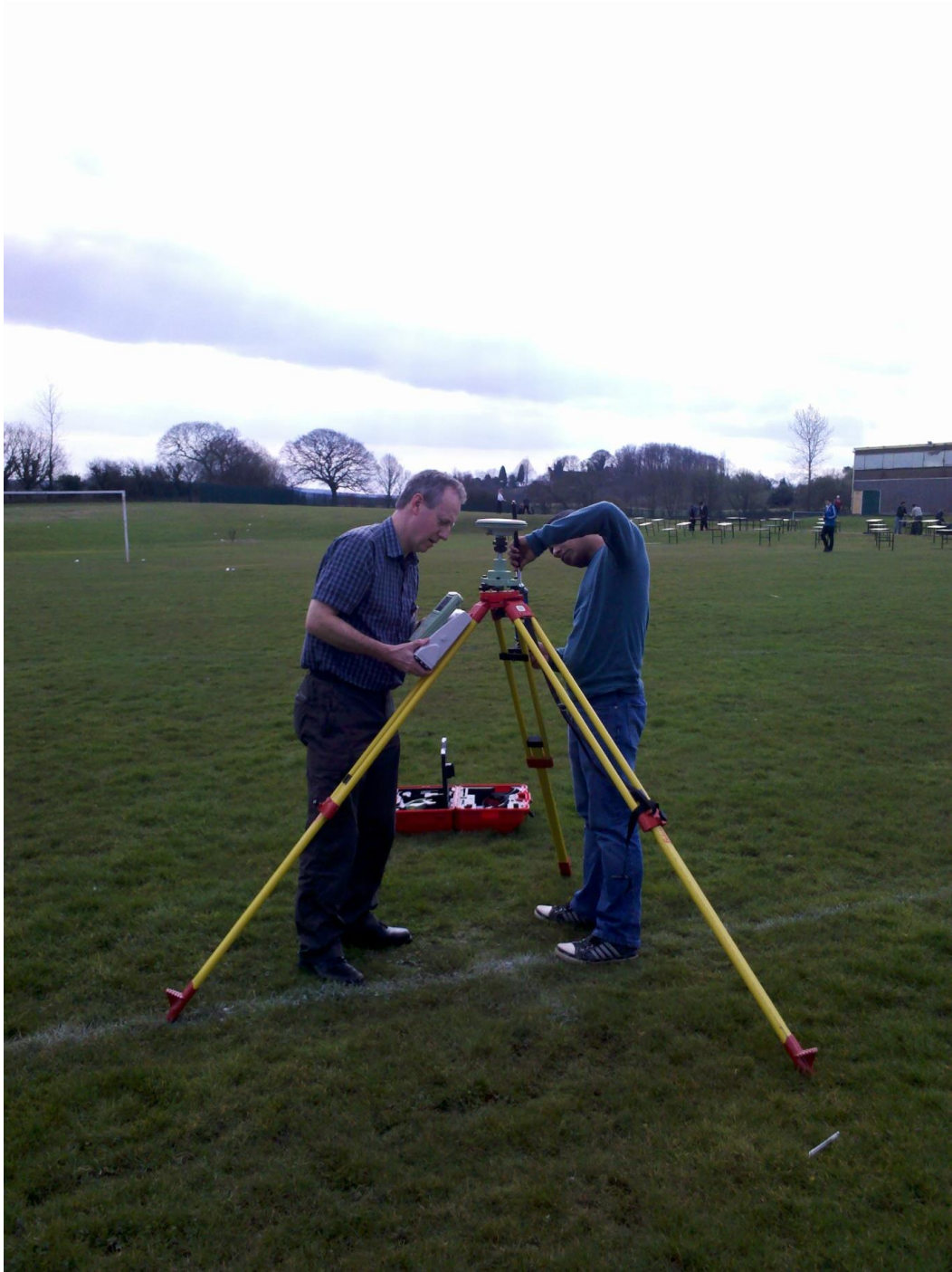
Figure 4-6 Leica GNSS base station set up for differential processing of the flights. Note the tables in the background showing the very short baseline used in processing.
