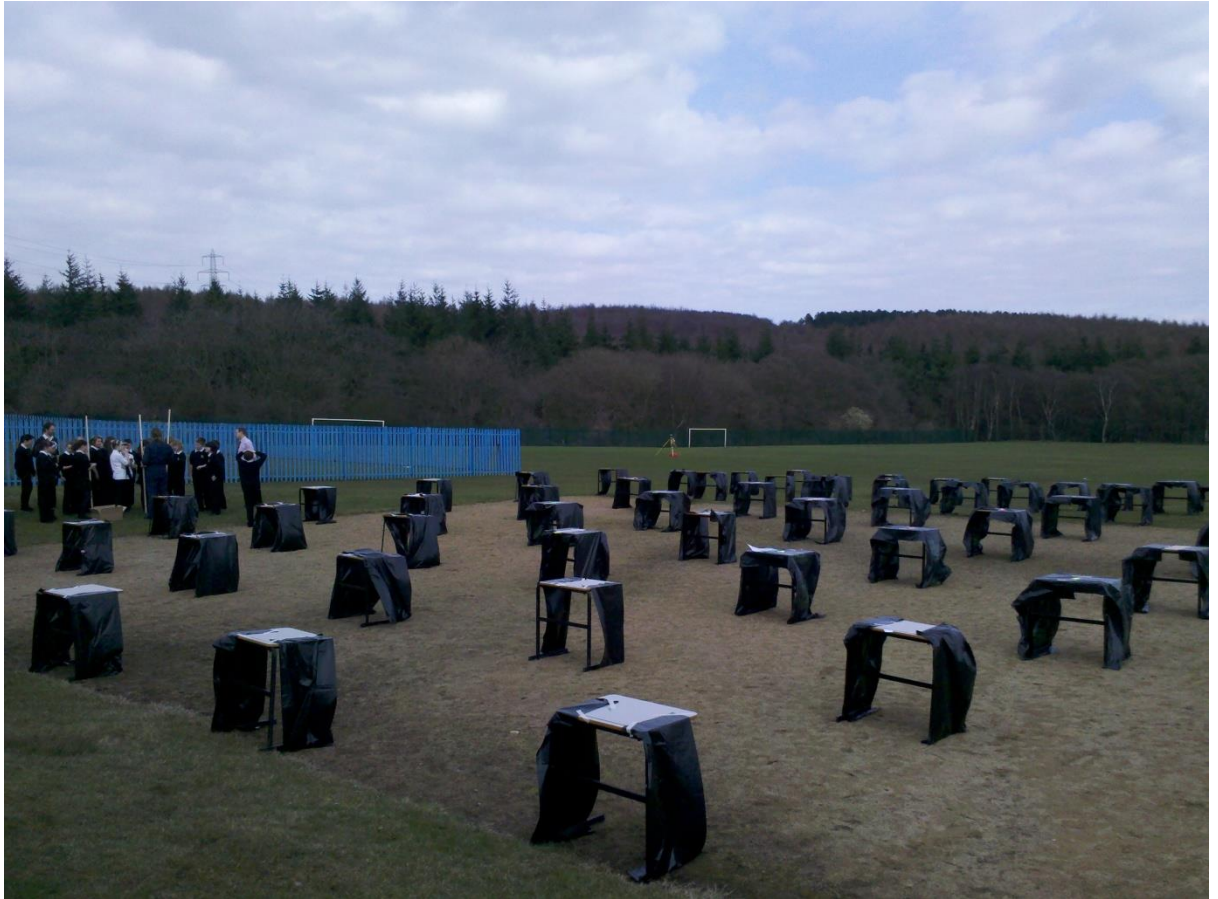
Figure 4-7 showing the tables with polythene wrapped around to prevent laser strikes under the table legs
