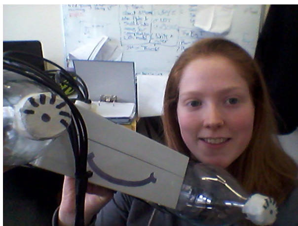
Figure 3.18: Floating bluetooth device for remote measurement and logging of temperatures in water
