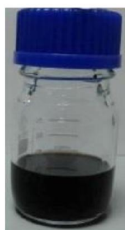
Figure 5.32: Black precipitate observed from sucrose crystal dissolution methodology for 2 mg/g sucrose crystals in 50 \mu\text{l/g} sulfuric acid microemulsion.
