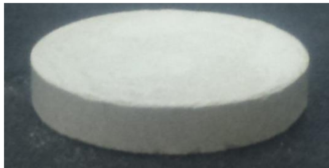
Figure 9. Artificial Na-bentonite core prepared by hydraulic press
