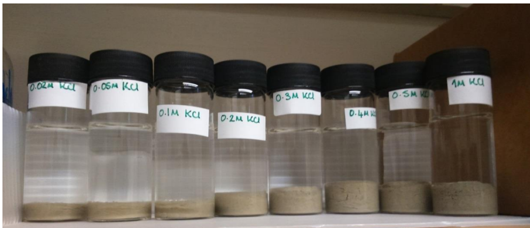
Figure 12. Application of equilibrium swelling tests
