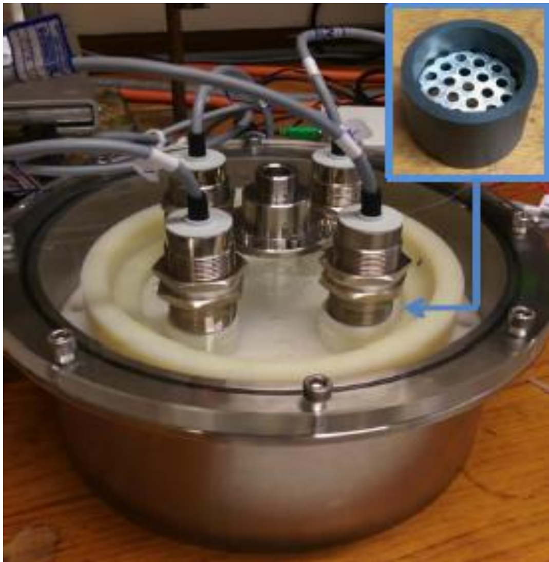
Figure 11. The non-contact linear displacement meter (NC-LDM). Inset photograph shows the sample holder along with the perforated metal disk the clay cores are placed on.
