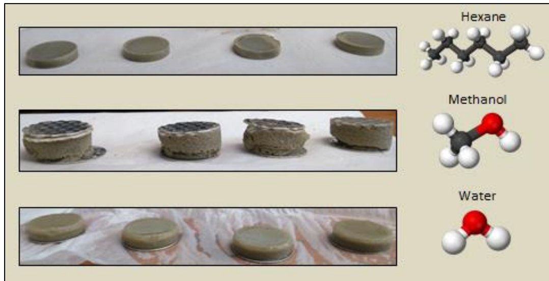
Figure 18. Photographic images of Na-bentonite cores after short term swelling tests in hexane, methanol and water.
