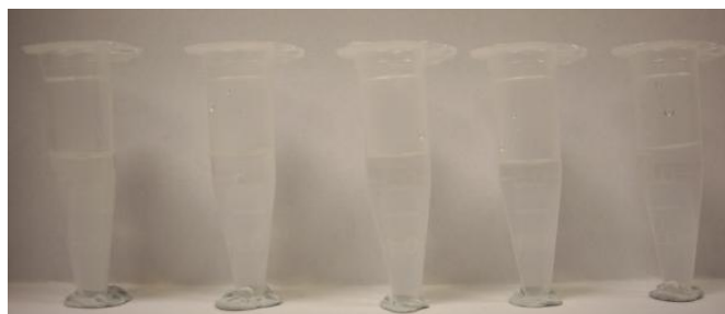
Figure 6-10: Ribonucleoside/purified SWNTs supernatant in water after sonication and centrifugation: Dispersion from left to right: adenosine/purified SWNTs, guanosine/purified SWNTs, thymidine/purified SWNTs, cytidine/purified SWNTs, and uridine/purified SWNTs.
