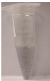
Figure 7-54: The mixture of aqueous dispersion of adenosine/GO and thymidine/GO after 2 min shaking.
